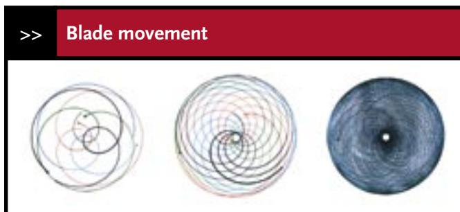
Figure 3. In a double planetary mixer, the orbital motion of blades is both predictable and efficient.
